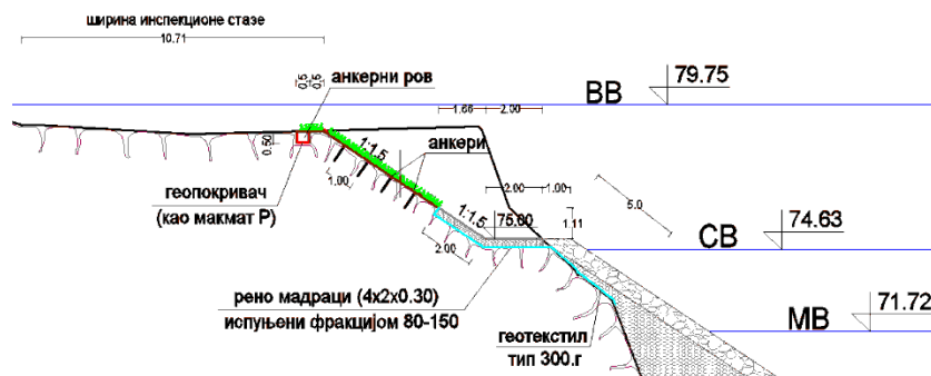
Figure 27: typical details of river bankal fortification - TYPE 1
